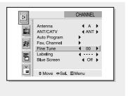
Move the joystick to the left or right to adjust the fine tuning.
